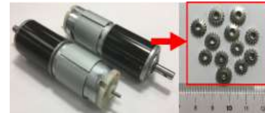
Carburized and tempered micro gears (applied to Tesla car door handles)
